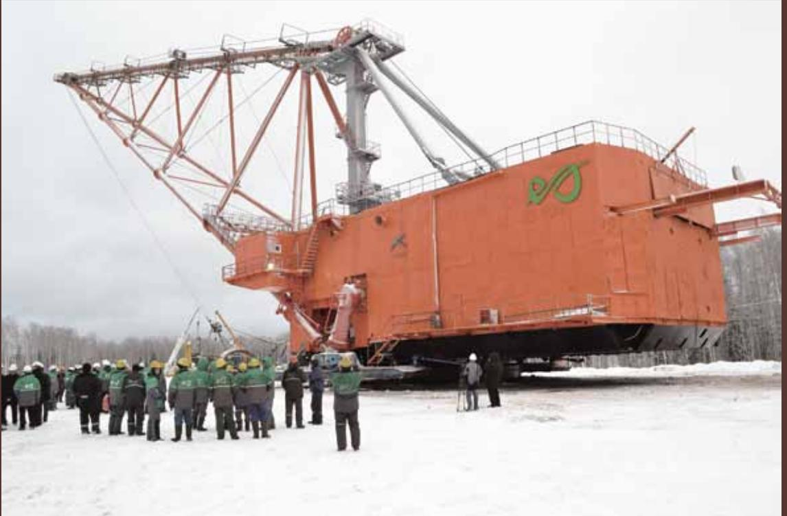
The machinery used for mining oil shale is unique and massive. For instance, two 2000-tonne walking excavators – “Aidu Pääsuke” (“Aidu Swallow”) (pictured) and “Aidu Sookurg” (“Aidu Crane”) – have gone down in the annals of technology, the operations to re-locate them from the Aidu pit to the Narva pit being unique in Europe in terms of their scale.
