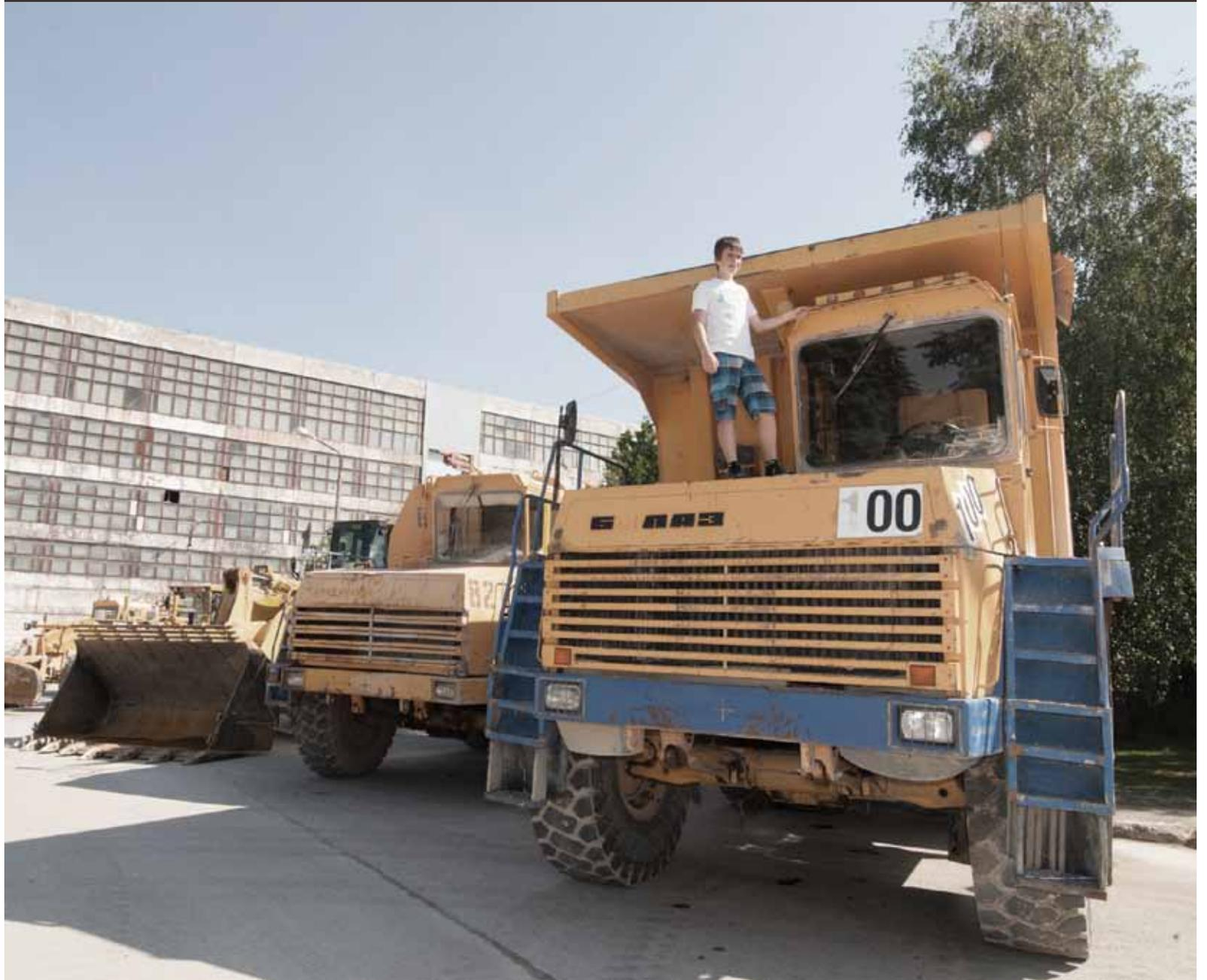
Transporting oil shale under various circumstances requires large, robust machinery. So, for instance, Estonian oil shale pits employ dump trucks with average load bearing capacities of 55 tonnes. Pictured is one such BelAZ mining dump truck.
